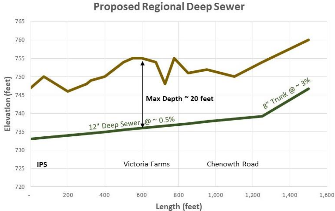
Figure 2. Proposed Deep Sewer Profile
